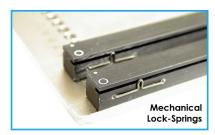
The StripFeeder .mod (Modular) System Version 2 now features a mechanical lock-spring to hold the tape in place by the sprocket hole for part registration and repeatable pick-and-place applications. This means you only have to teach the pick-up location one time and you can consistently reload the unit with the same parts over and over for longer runs. This feature is compatible with both paper and emboss tapes.
